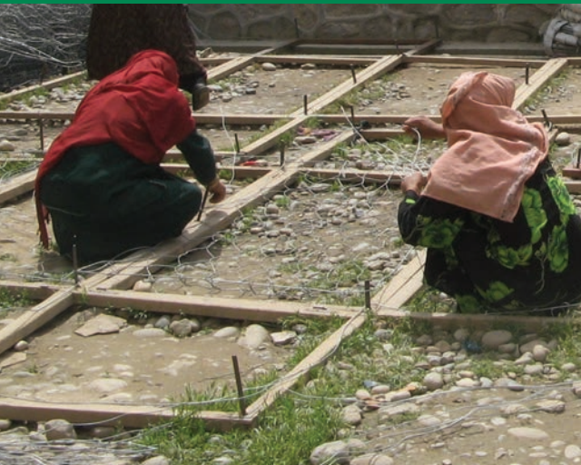
Women making gabion baskets, Afghanistan Photo credit: Social Protection Directorate, MRRD, Afghanistan
